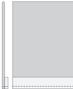
made-up fabric, flat welt 12 mm
